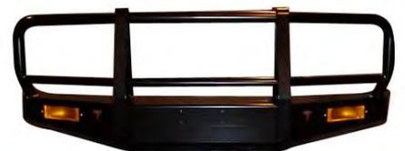
Bull bars must be free of sharp protrusions and all exposed sections of the bull bar and fittings must be radiused and deburred. Forward and side members should be designed to reduce the risk of injury to any person who may come into contact with the bull bar.
