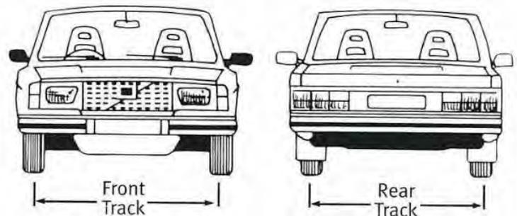
The wheel track of off-road four wheel drive vehicles and goods vehicles must not be increased by more than 50mm beyond the maximum specified by the vehicle manufacturer for the particular model. If a solid axle from another manufacturer is used, the wheel track may be increased by 50mm beyond the maximum specified by the vehicle manufacturer for that particular axle, provided all other requirements such as clearances are met and the tyres do not protrude outside of the vehicle bodywork.
